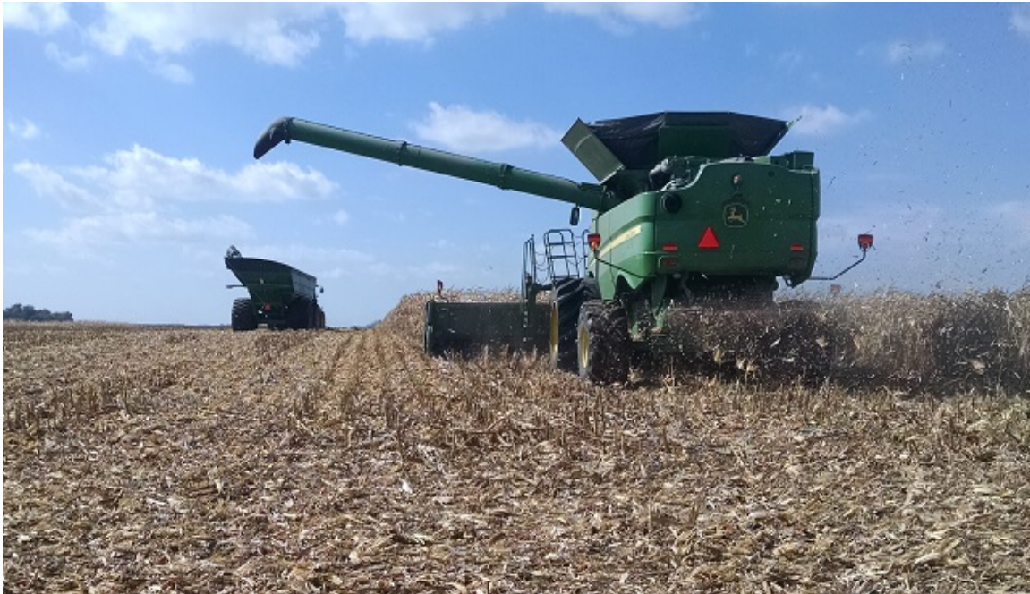
Figure 3 – Harvesting corn. The combine will off load corn on the go into the waiting dump cart allowing no interruption of harvesting.
