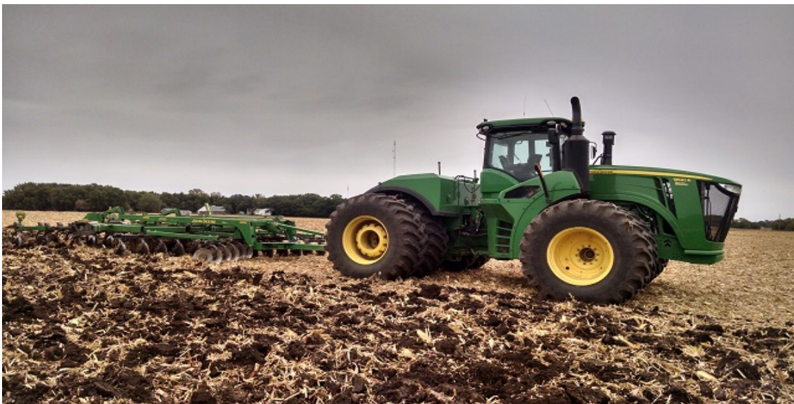
Figure 4 – Deep ripping of corn stubble after harvest. This will be the first operation to get this field ready for soybeans in 2019.
