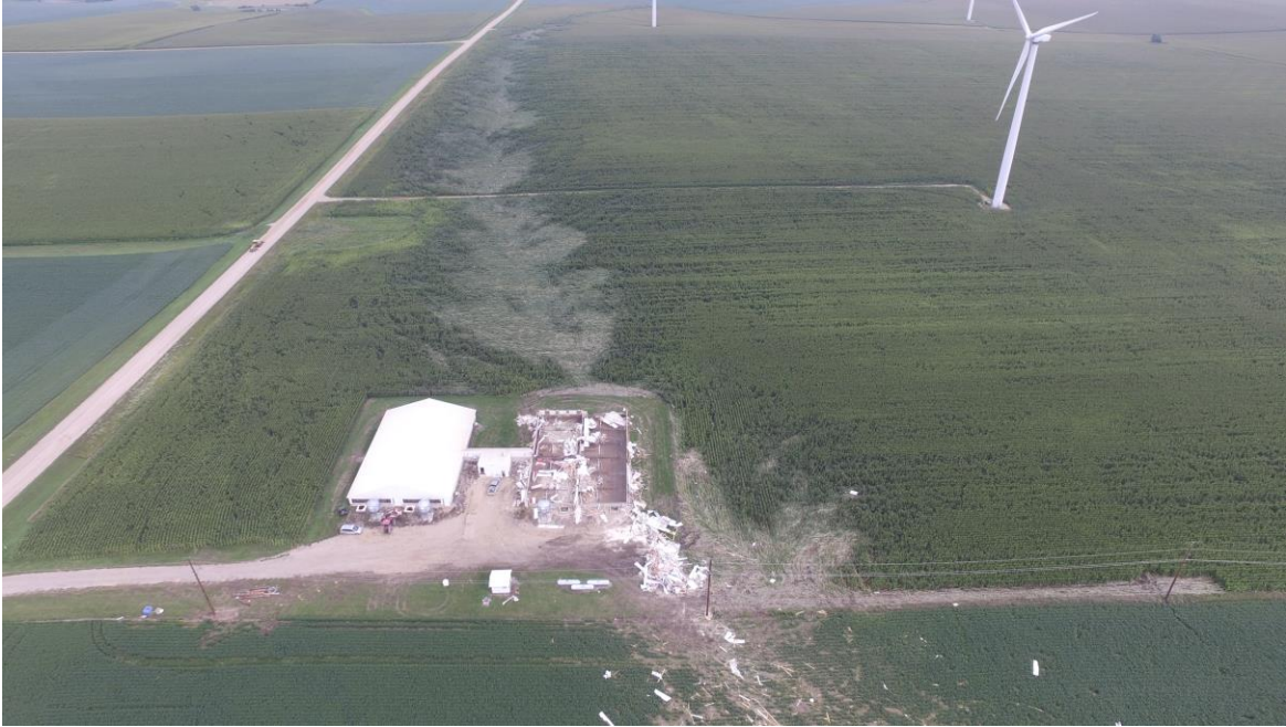
Figure 1 – This picture taken near Rushmore shows damage to crops and the total destruction of a hog barn from the tornado on August 18th. The hog barn to the left was unharmed.
