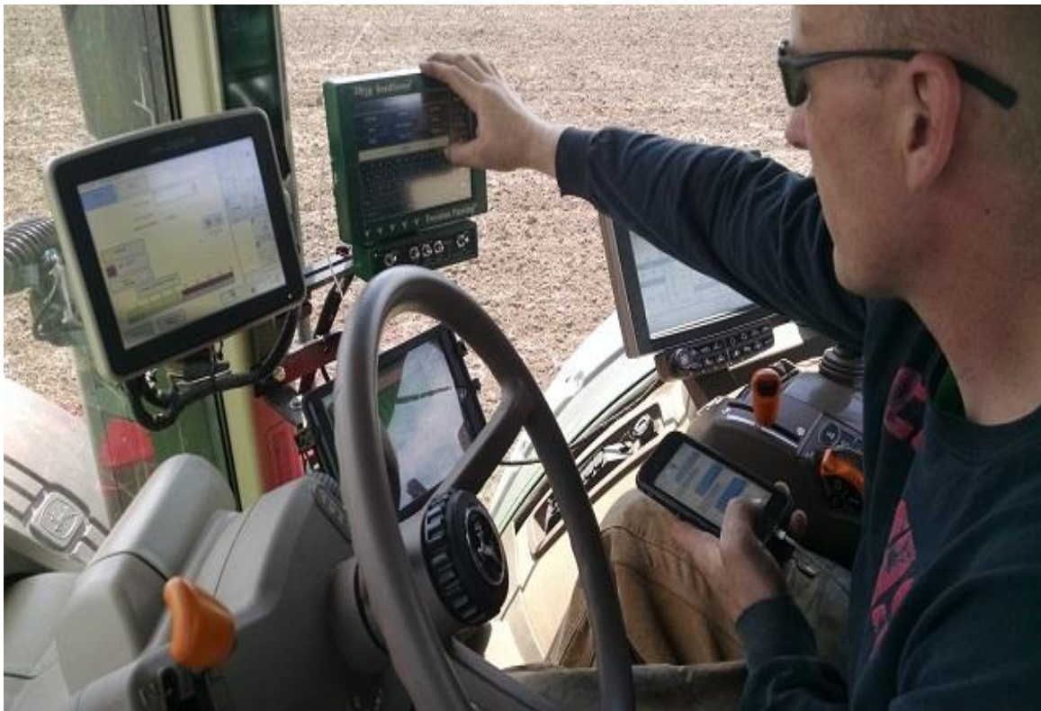
Figure 4 – Technology continues to drive the planting process. A screen overload? Electronic and electrical devices monitor and regulate planting population, down pressure (compaction), ground speed, application rates of liquid fertilizer and herbicide, seed spacing, statistical data, varietal placement and etc. all on a row by row and GPS site specific basis. The technology can even be used to input prescriptions based on soil type and varieties.
