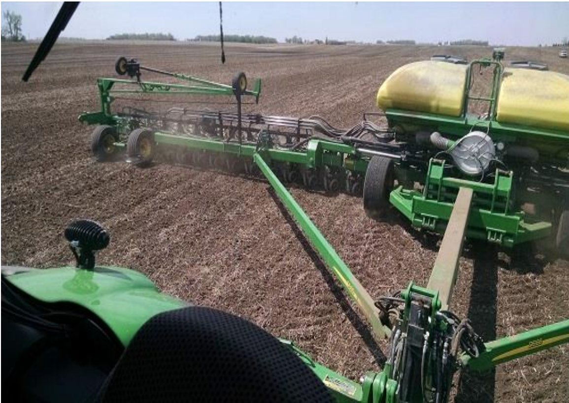
Figure 3 – A view of corn planting from the cab of the tractor. Monitors with indicators and alarms are extremely important for the planting process, but so is the human eye and getting out of the tractor and digging up some seeds from time to time.
